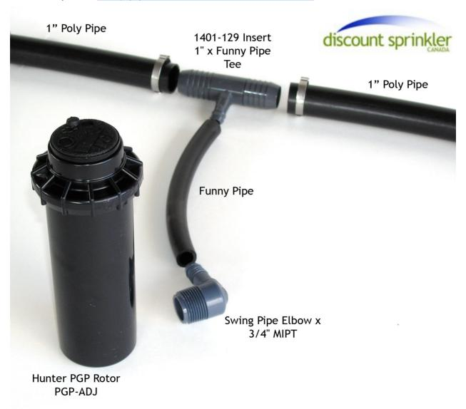
Attaching a rotor at the end of a run of poly pipe is basically the same as the assembly in the middle of a run on the previous page. The only difference is that instead of a tee you would use a 1429-129 Funny Pipe Coupler (or Adapter).
