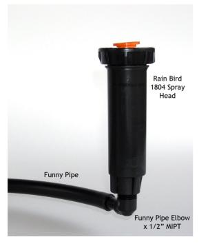
The method of installation is the same as a rotor zone except for the fitting that connects the funny pipe to the bottom of the sprinkler head. Most spray heads (Rain Bird 1800 and Hunter Pro-Spray) have a 1/2" female inlet on the bottom which means that the funny pipe elbow needs to have a 1/2" male thread on the end that connects to the sprinkler.
